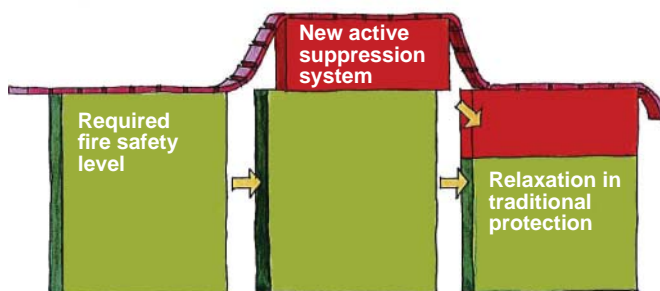
Principle for fire safety design by sprinklers: Increased fire safety by installation of sprinklers may lead to relaxations in the passive fire means, and still fulfil the same or higher safety level.
